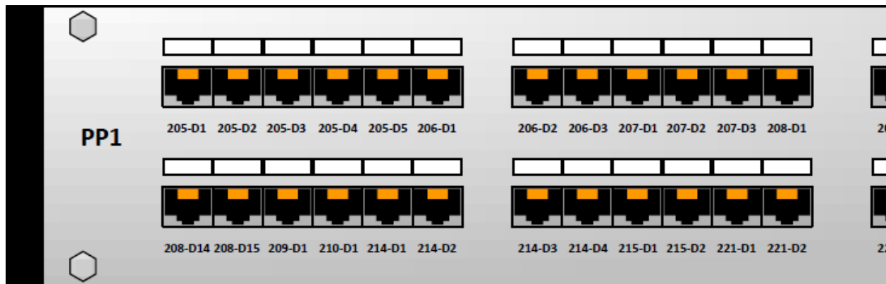
Figure 2-3. Copper Patch Panel Label – Example
